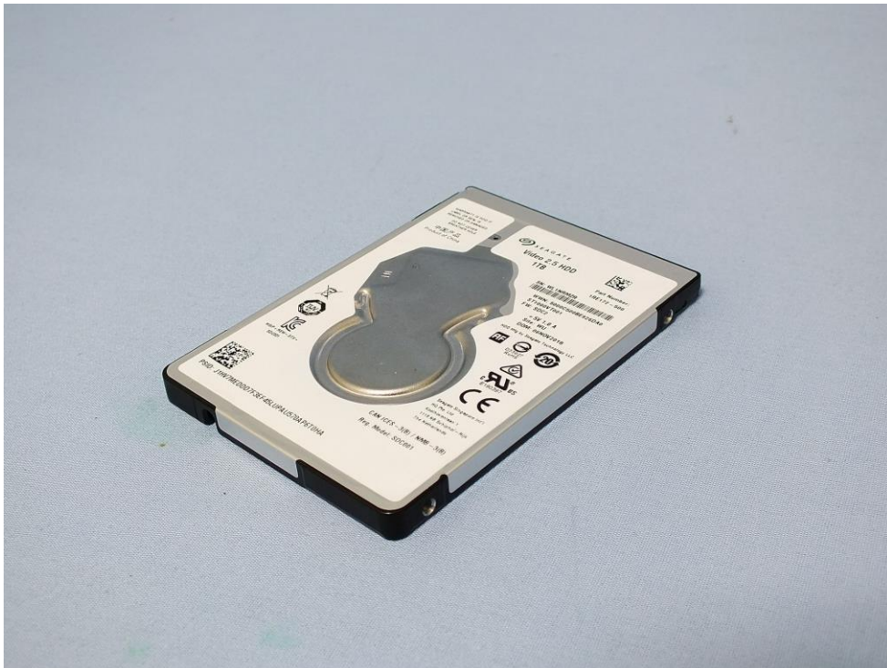
HDD (Brand: SEAGATE, Model: ST1000VT001)
