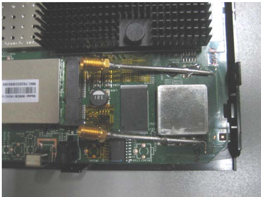
ARRIS IP815 SAMPLE 1621-04 (INTERNAL SHOWING SMA CONNECTORS)
