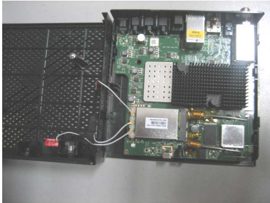
ARRIS IP815 SAMPLE 1621-04 (INTERNAL SHOWING MODIFIED ANTENNAS)
