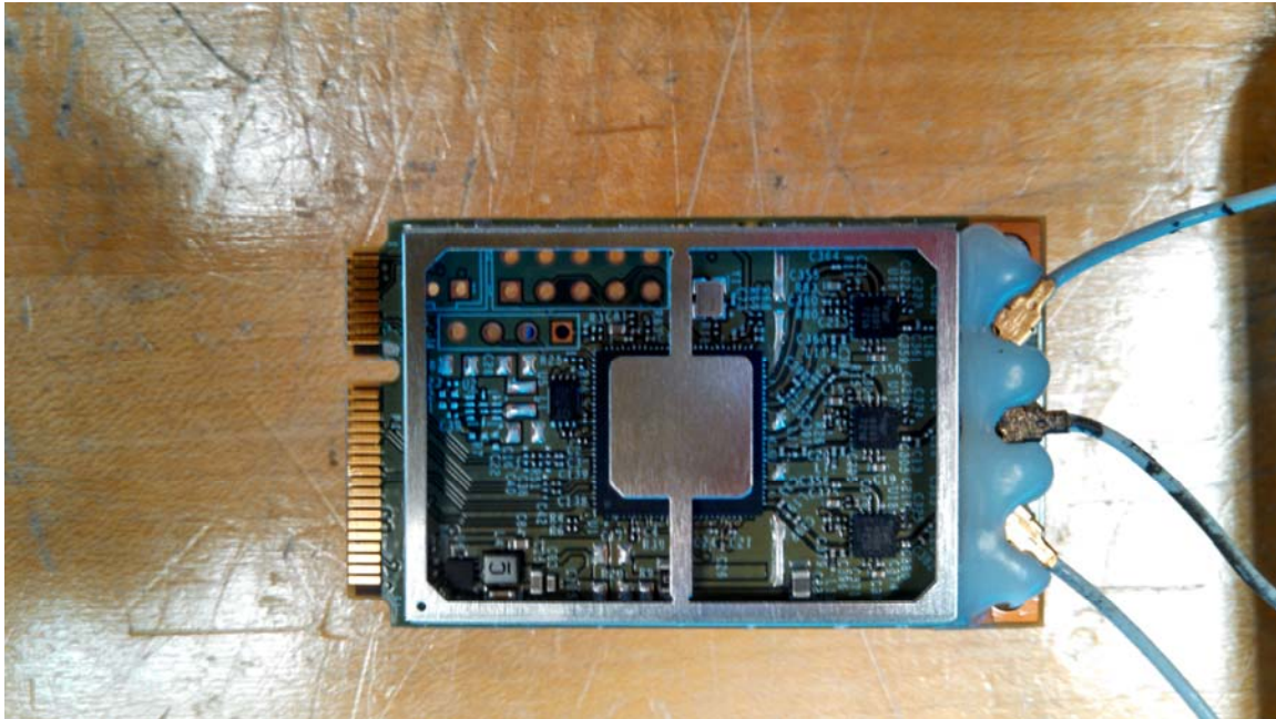
RADIO BOARD TOP SHIELD REMOVED
