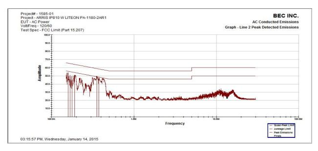
**Results:** All conducted emissions measured on the telecommunications port(s) of the LITEON Model PA-1180-2AR1 supply are below the limits specified in FCC Section 15.207 by a margin of at least 7.9 dB.
