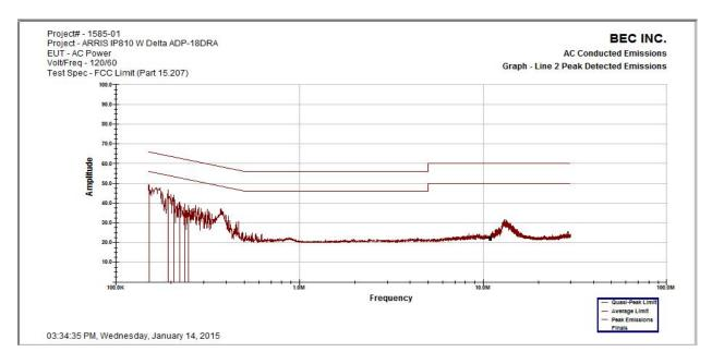
**Results:** All conducted emissions measured on the telecommunications port(s) of the Delta Model ADP-18DRA supply are below the limits specified in FCC Section 15.207 by a margin of at least 19.5 dB.
