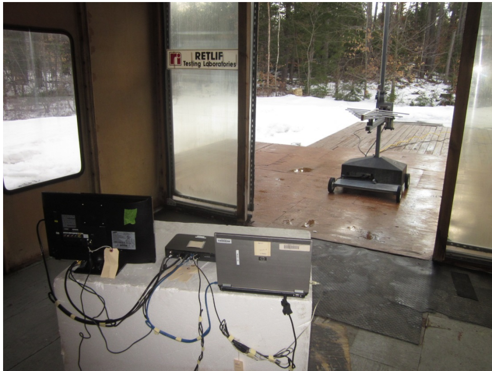
Horizontal Antenna Polarization, 200 GHz to 1 GHz
