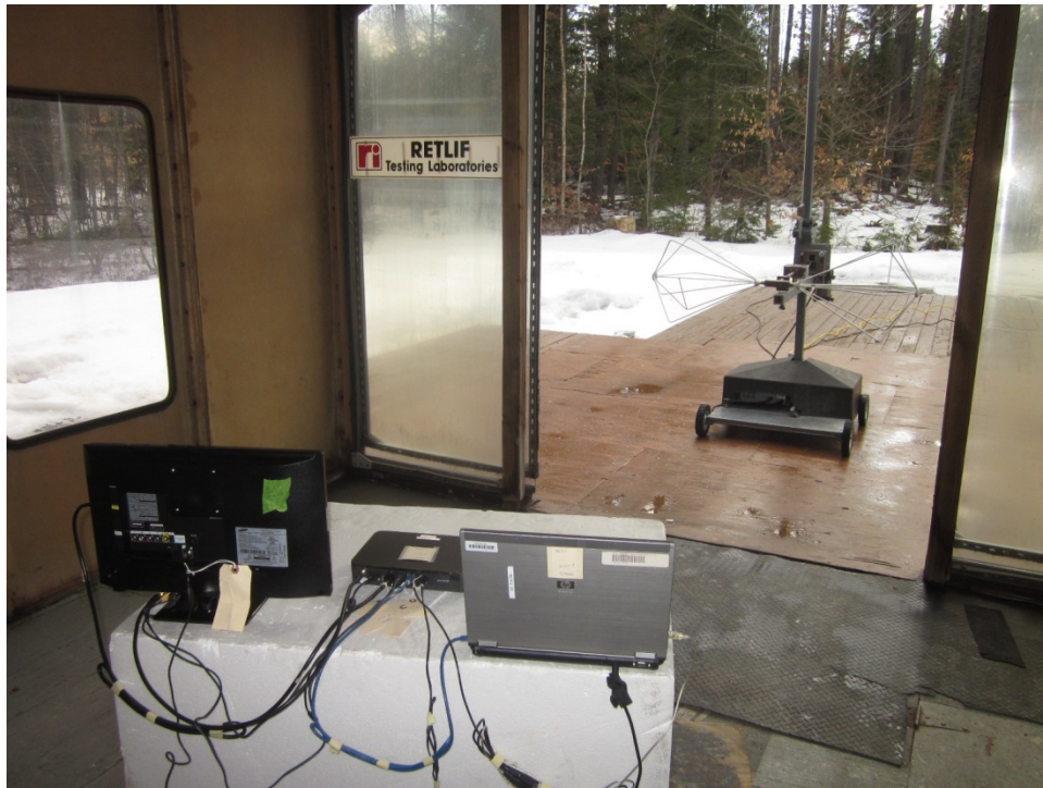
Horizontal Antenna Polarization, 25 MHz to 200 MHz
