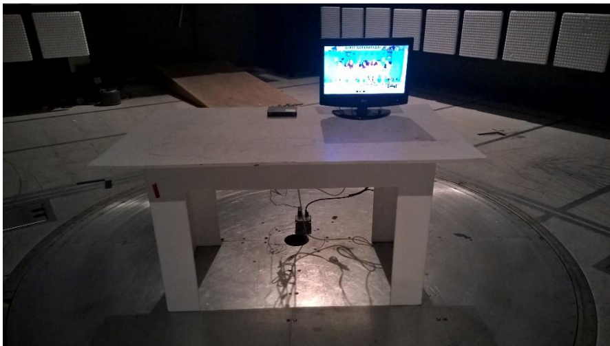
Figure 15.1-4: Radiated disturbance setup photo
