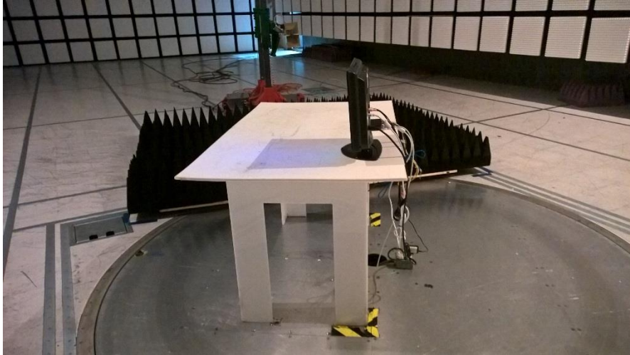
Figure 15.1-5: Radiated disturbance setup photo above 1GHz
