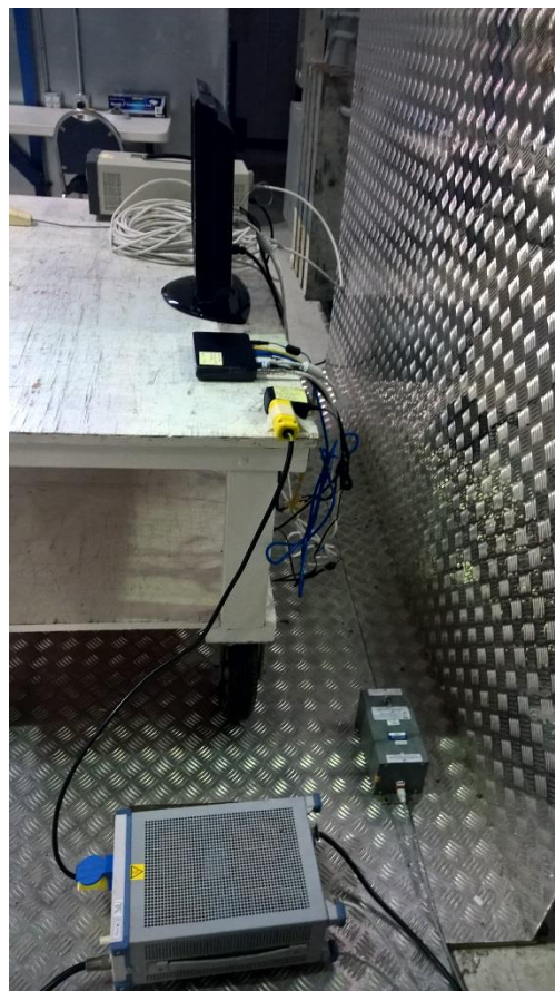
Figure 15.2-4: Conducted disturbance at mains port setup photo
