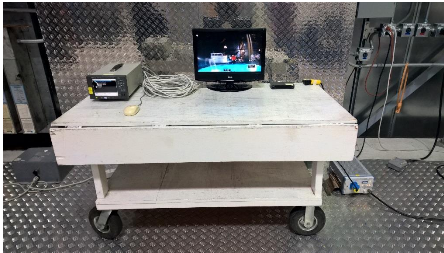
Figure 15.2-3: Conducted disturbance at mains port setup photo
