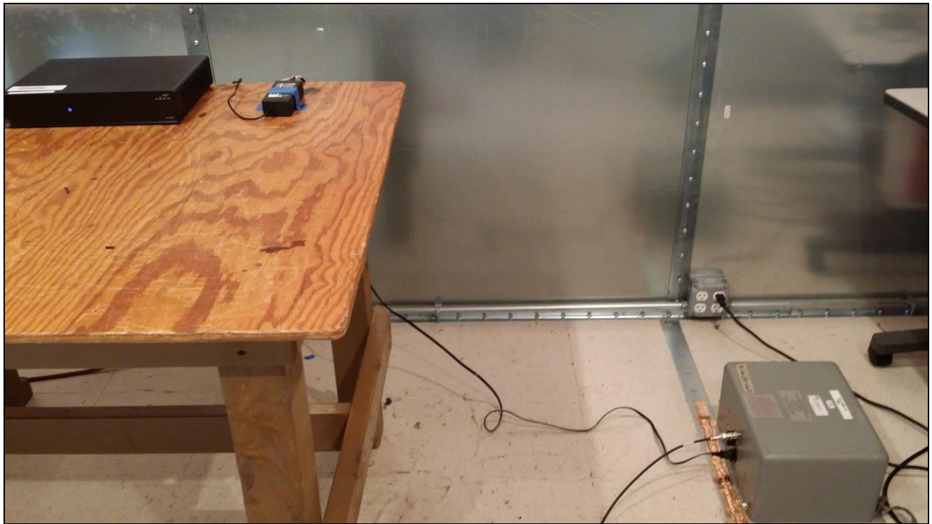
Photograph 1. Conducted Emissions, 15.207(a), Test Setup
