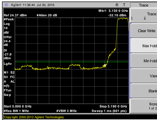
Plot 129. Band Edge, 802.11ac 20 MHz, MIMO, Channel 36, Peak
