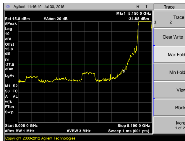
Plot 143. Band Edge, 802.11ac 20 MHz, SISO, Channel 36, Peak
