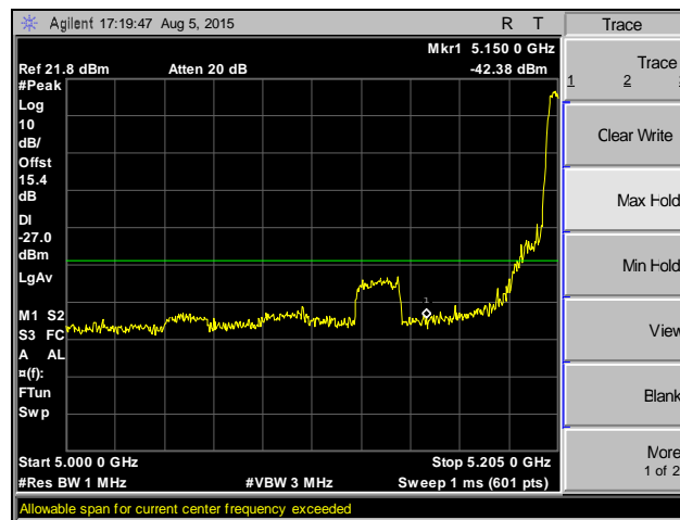
Plot 149. Band Edge, 802.11ac 20 MHz, SISO, Channel 42, Peak
