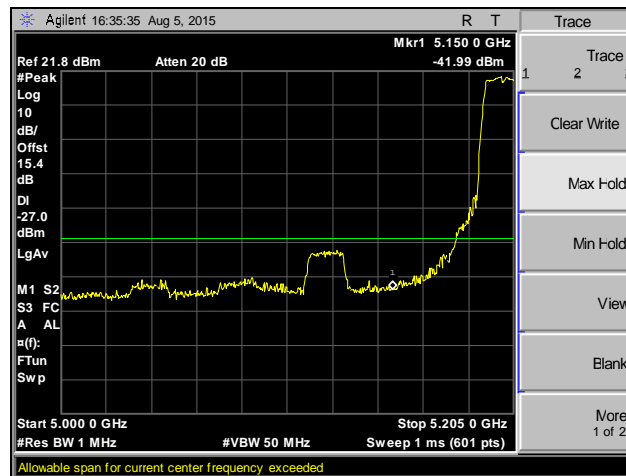
Plot 119. Band Edge, 802.11a 20 MHz, SISO, Channel 40, Peak
