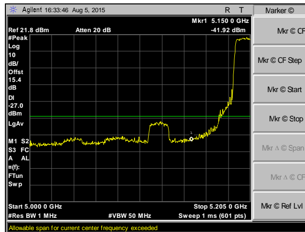
Plot 147. Band Edge, 802.11ac 20 MHz, SISO, Channel 40, Peak
