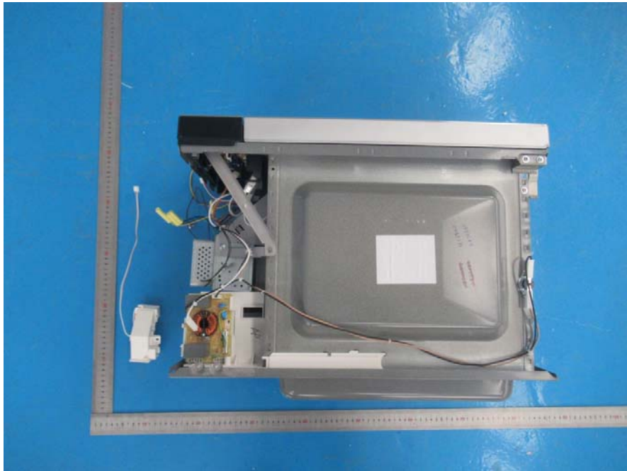
EUT – Cover off View -5
