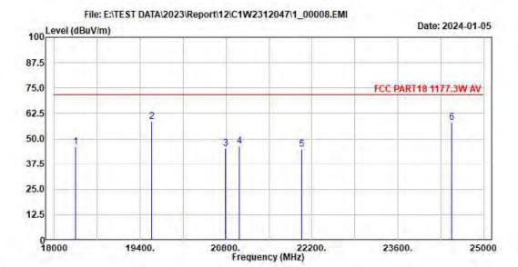
Site NO. : NO.2 3M Chamber Instrument 1 : Spectrum N9030A(217)
