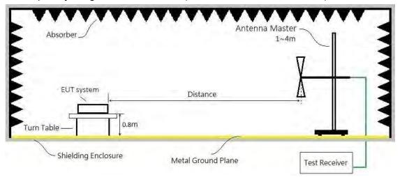
For frequency range above 1GHz (at Semi-Anechoic Chamber)
