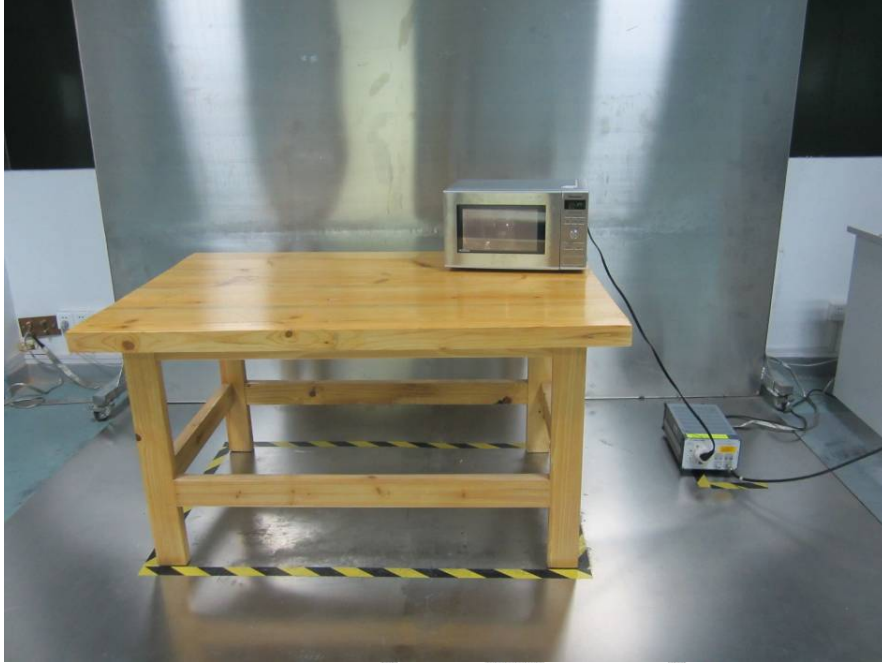
Conducted Emissions - Front View
