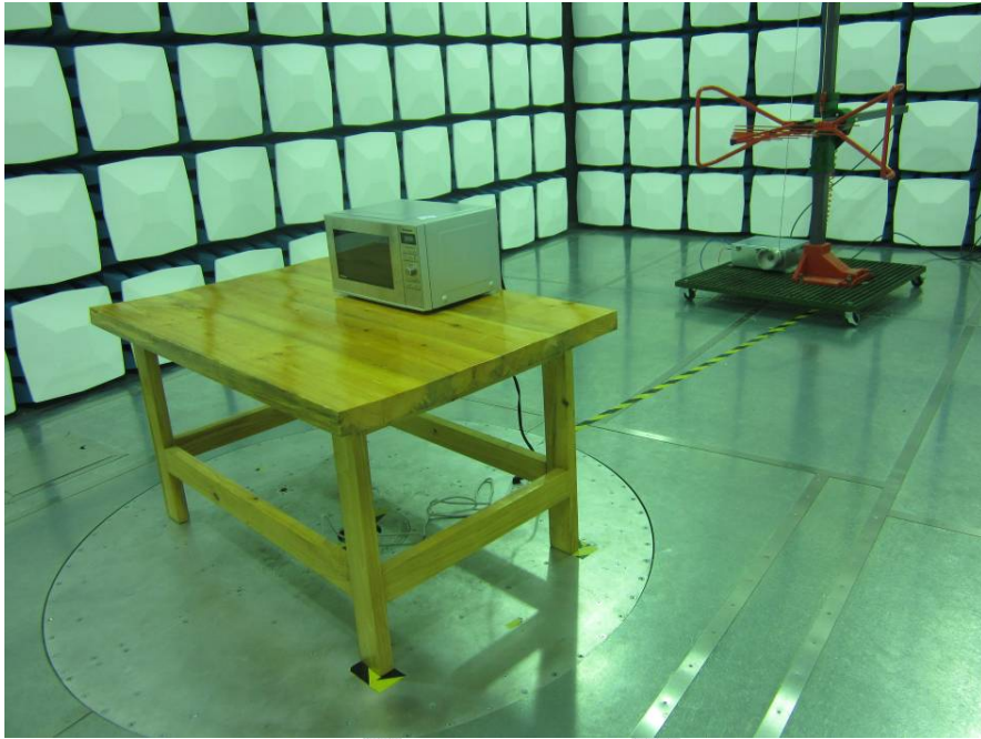
Radiated Emissions - Front View (30 MHz-1 GHz)
