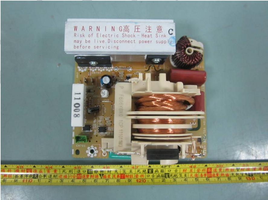
EUT – Power Supply Board Top View
