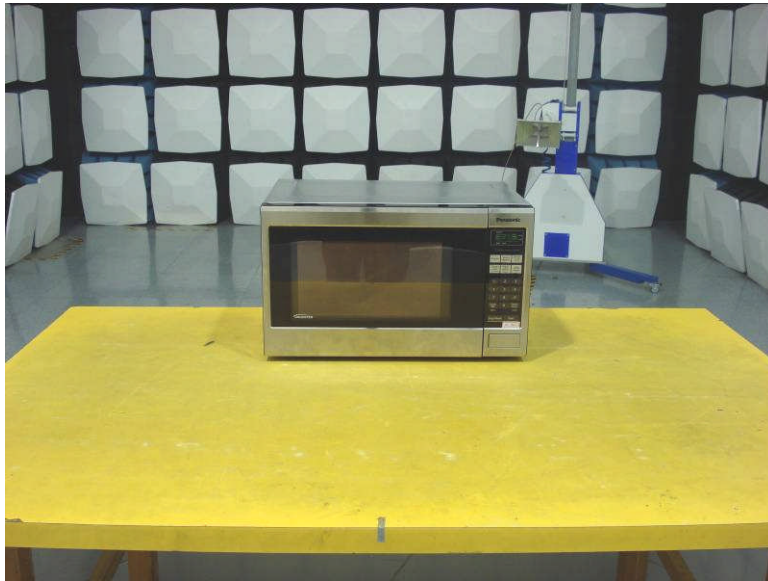
Radiated Emissions - Front View (Above 1 GHz)
