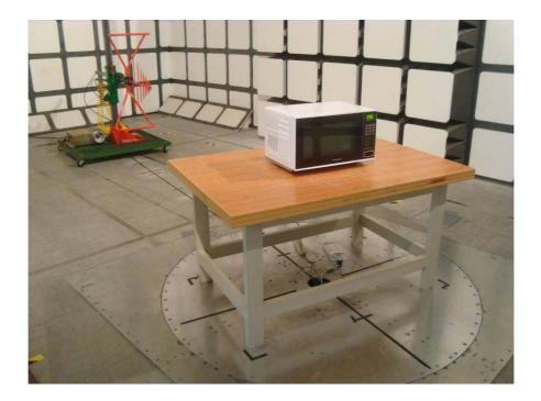
Radiated Emissions - Front View (30 MHz-1 GHz)
