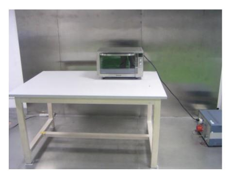
**30MHz to 1000MHz: Radiated Emission - Front View**
