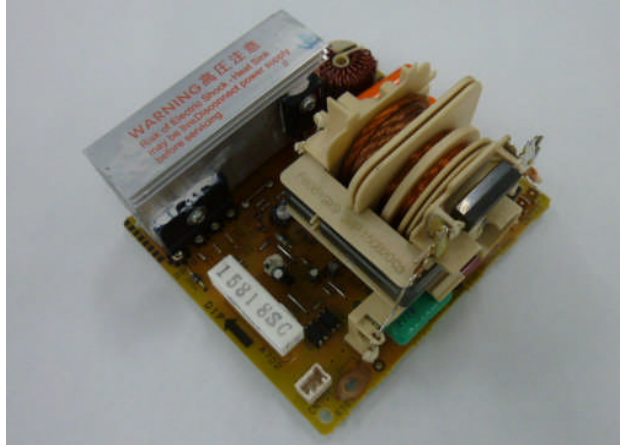
View of Power Inverter
