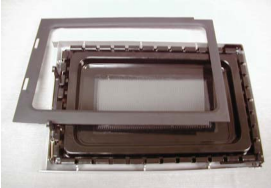
Exhibit 2-K View of Door Choke Construction
