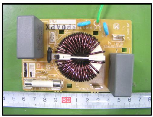
**EUT - Filter Board Circuits View**
