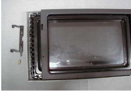
Exhibit 2-L View of Door Choke Construction
