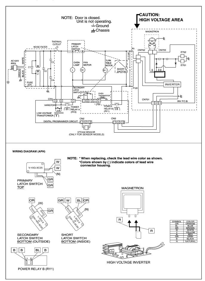
**EXHIBIT C: Schematic Diagram (Inverter Power Supply)**
