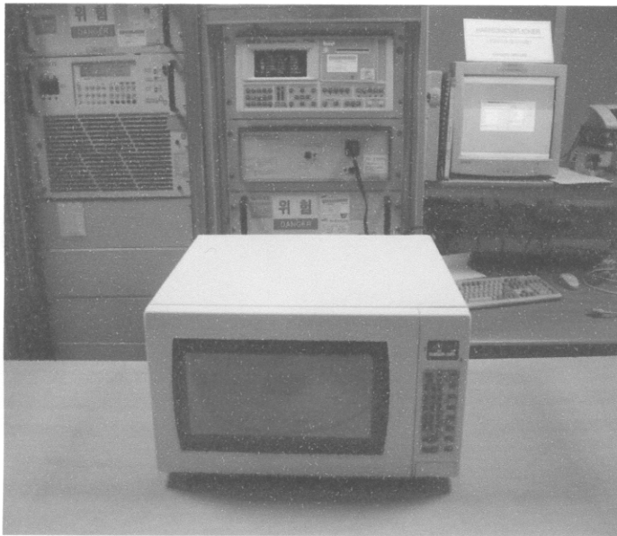
Fig.3 Test Setup for RF output power
