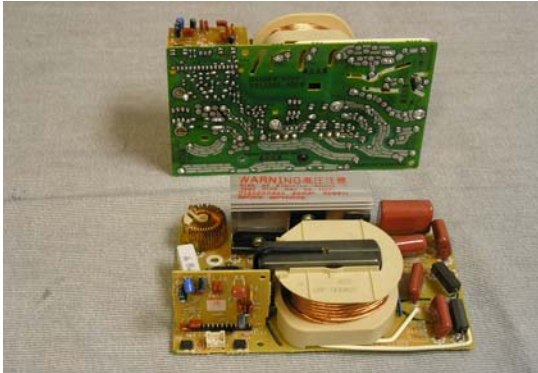
Exhibit 2-K View of Inverter Circuitry
