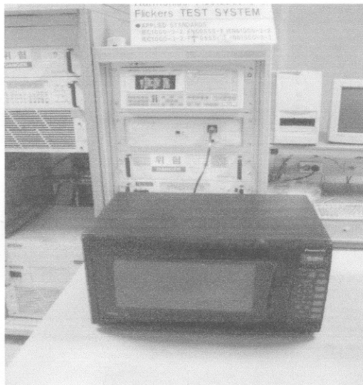
Fig.3 Test Setup for RF output power
