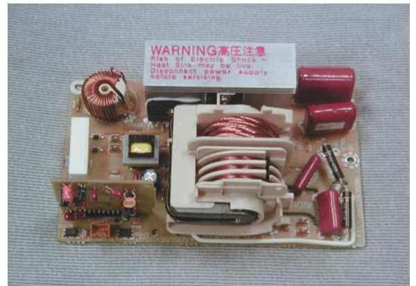
Exhibit 2-K View of Inverter Circuitry
