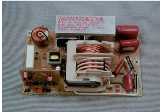
Exhibit 2-K View of Inverter Circuitry
