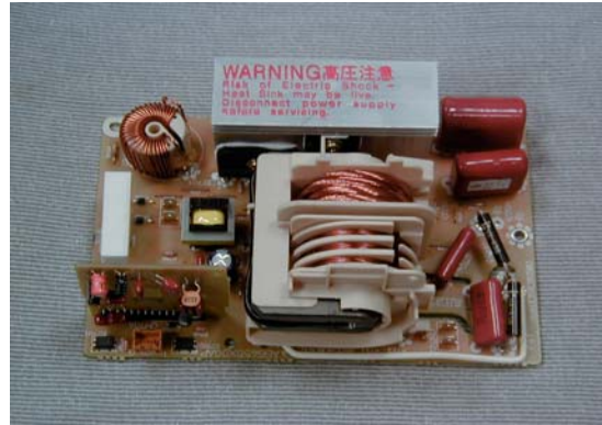
Exhibit 2-K View of Inverter Circuitry
