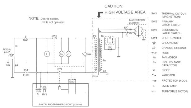
IMPORTANT SAFETY NOTICE: POTENTIALS ABOVE 120V IS PRESENT ON THE PARTS AND WIRING IN SECONDARY CIRCUIT OF HIGH VOLTAGE TRANSFORMER. V/HEN OVEN IS ENERGIZED. EXTREMELY CARE SHOULD BE TAKEN DURING REPAIR.
