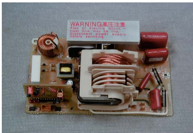
Exhibit 2-K View of Inverter Circuitry
