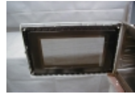
Exhibit 2-H, View of Door Construction Illustrating integral choke
