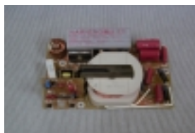
Exhibit 2-J, View of Inverter Power Supply
