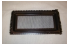
Exhibit 2-H, View of Door Construction, Illustrating Integral Choke
