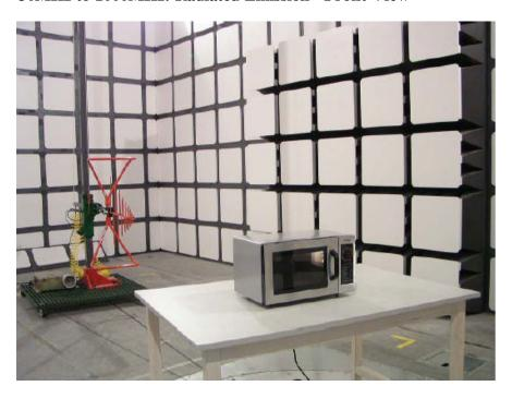
30MHz to 1000MHz: Radiated Emission - Rear View
