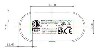
The marking information is located at the bottom of apparatus
