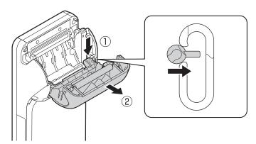
**3.** Raise (1) and close (2) the printer cover to insert the printer cover shafts into the bearings.
