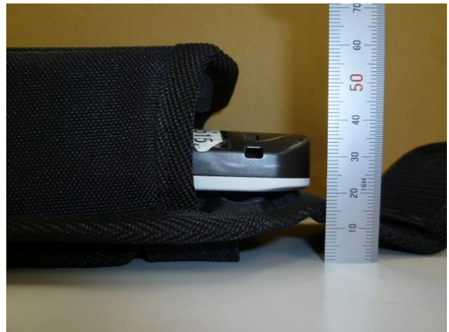
When the device attached the holster is away human body 20mm.
