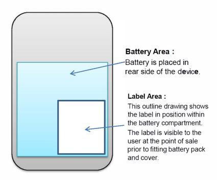
The label is located inside the battery lid (under the battery), and it is permanently attached by glue, so it is not easily removed from the device.
