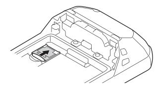
• To remove a microSD card, follow the same procedure, and then pull out the microSD card at step 3.
