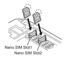
4. Close the Nano SIM card slot (1), and slide it in the direction of the arrow (2) until you hear a click.
