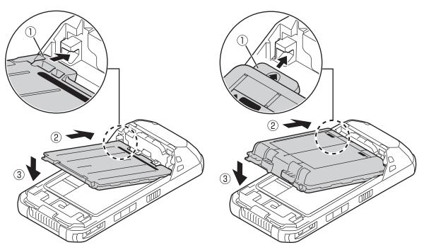
• The battery may protrude out of the unit even if you install the battery correctly. However, this is not a malfunction or defect.
