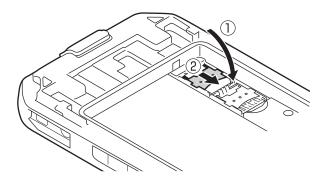
• To remove a SIM card, follow the same procedure, and then pull out the SIM card at step 3.
