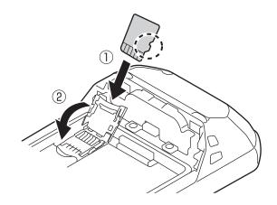
**4.** Slide the microSD card slot in the direction of the arrow until you hear a click.
