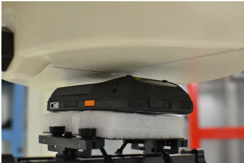
SAR Test Setup Photo 10 – Back Side at 1.0 cm with L-Battery
