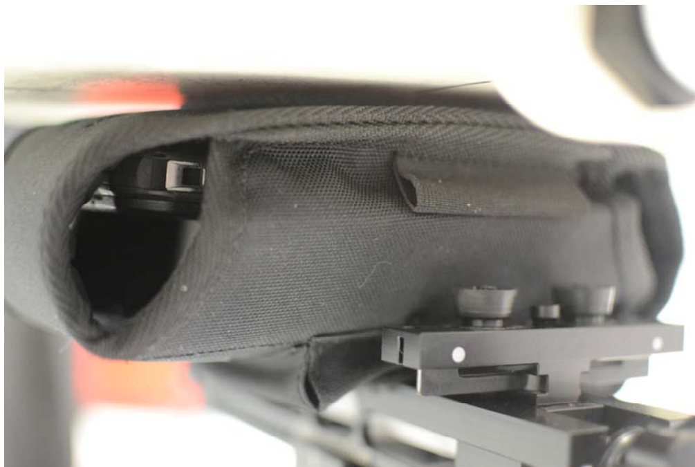
SAR Test Setup Photo 18 – Front Side at 0.0 cm with Standard Battery and Body Holster Accessory
