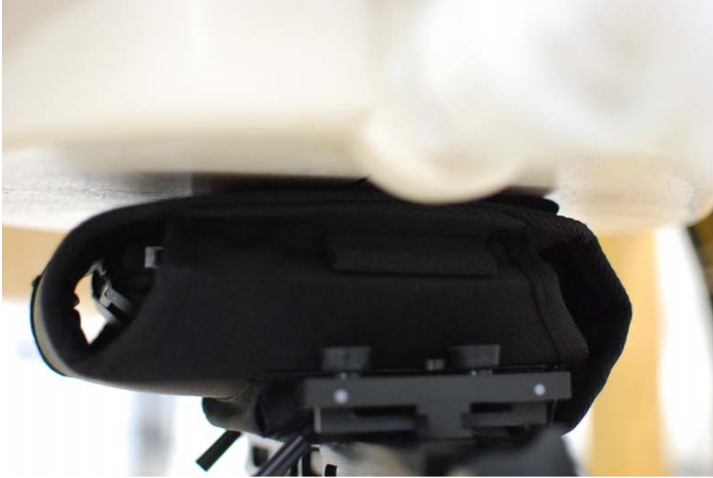
SAR Test Setup Photo 19 – Front Side at 0.0 cm with L-Battery and Body Holster Accessory
