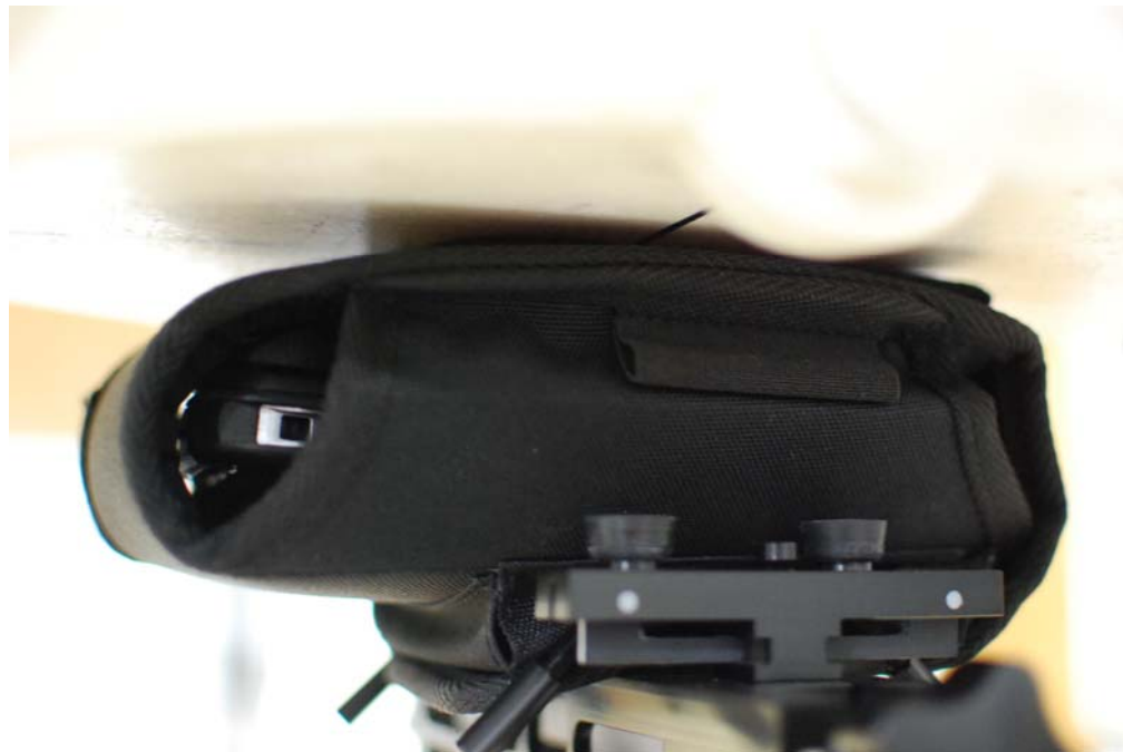
SAR Test Setup Photo 12 – Back Side at 0.0 cm with L-Battery and Body Holster Accessory
