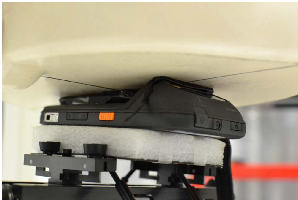
SAR Test Setup Photo 13 – Back Side at 0.0 cm with Standard Battery and Hand Strap Accessory
