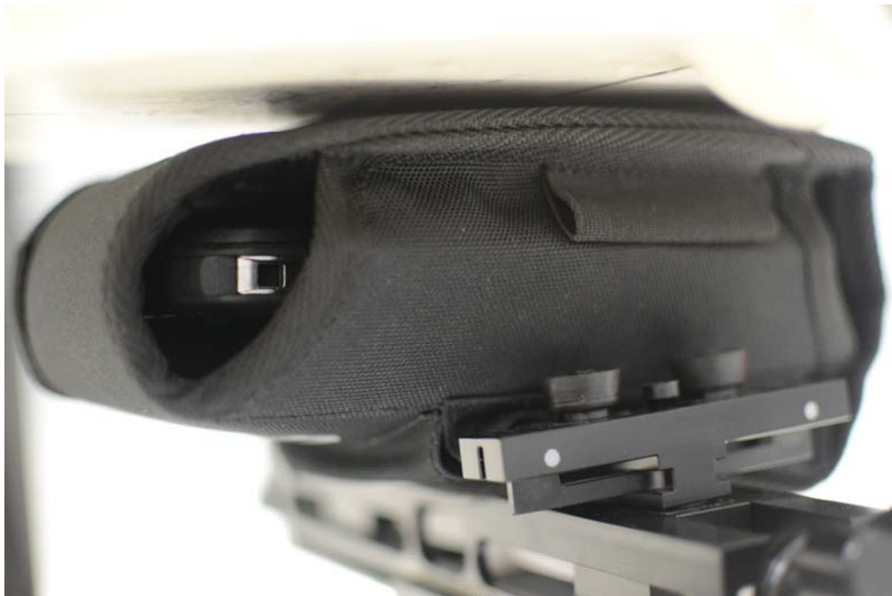
SAR Test Setup Photo 11 – Back Side at 0.0 cm with Standard Battery and Body Holster Accessory
