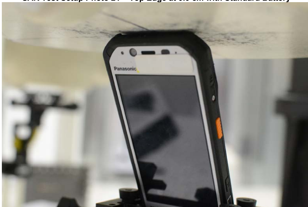
SAR Test Setup Photo 22 – Top Edge (Tilt) at 0.0 cm with Standard Battery
