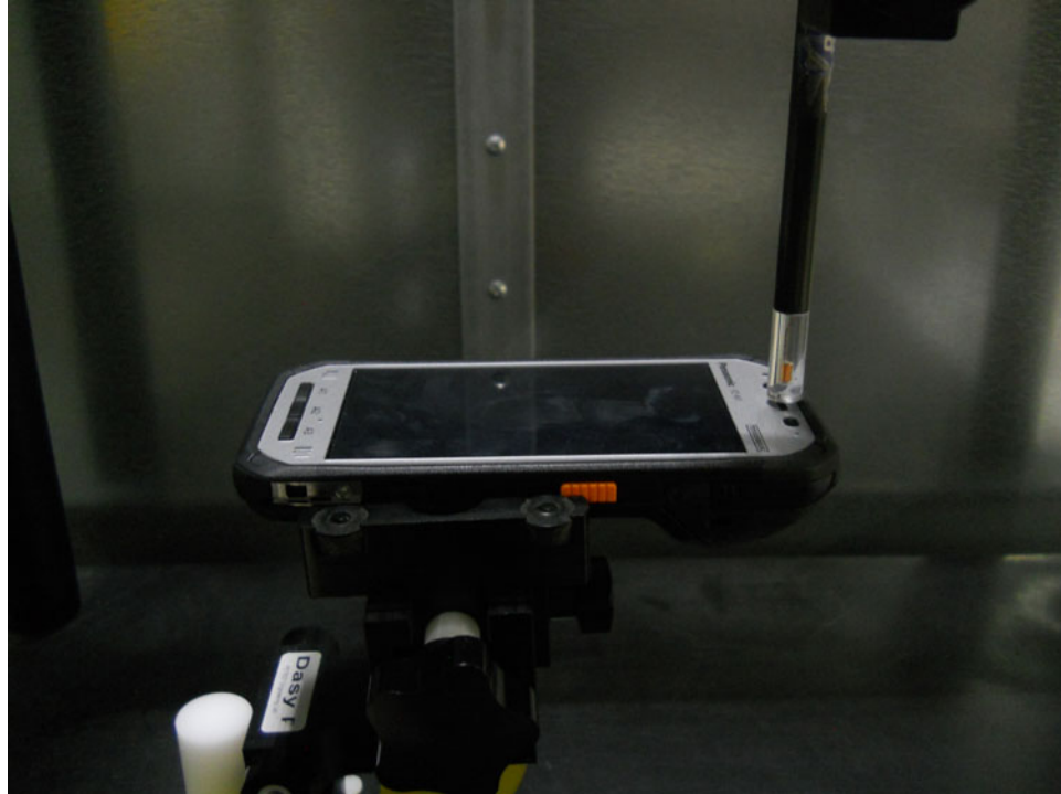
Figure 15-1 Test Setup for Wireless Device (Standard Battery)
