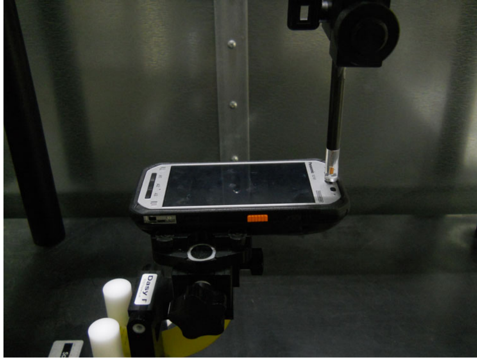
Figure 15-3 Test Setup for Wireless Device (L-Battery)
