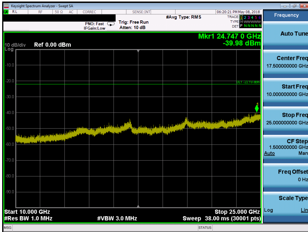
Plot 7-22. Conducted Spurious Plot (Bluetooth (LE), 1Mbps – Ch. 0)
