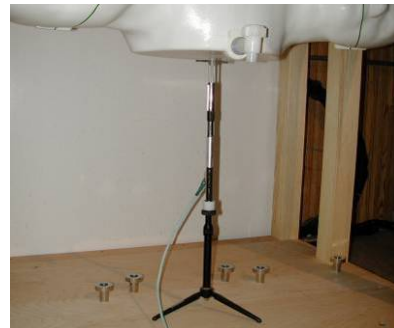
Figure 9-2 System Verification Setup Photo
