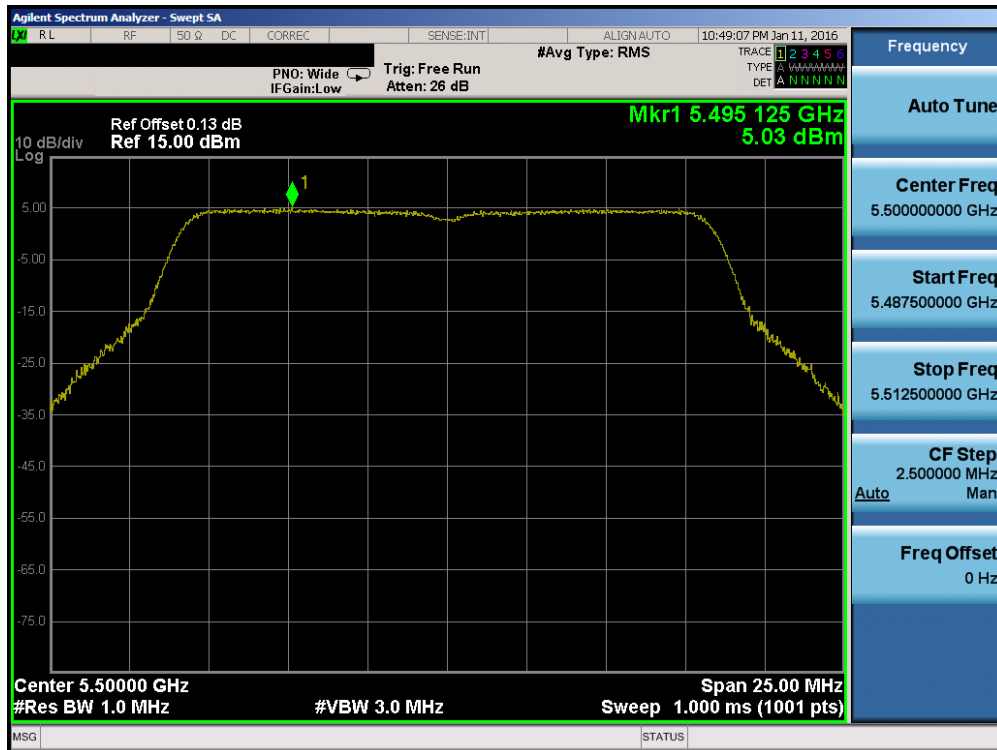
Plot 7-56. Power Spectral Density Plot (802.11a (UNII Band 2C) – Ch. 100)
