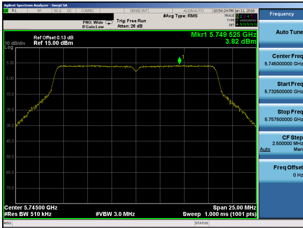
Plot 7-66. Power Spectral Density Plot (802.11a (UNII Band 3) – Ch. 149)
