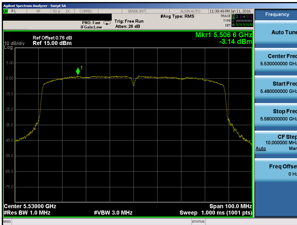
Plot 7-65. Power Spectral Density Plot (80MHz BW 802.11ac (UNII Band 2C) – Ch. 106)
