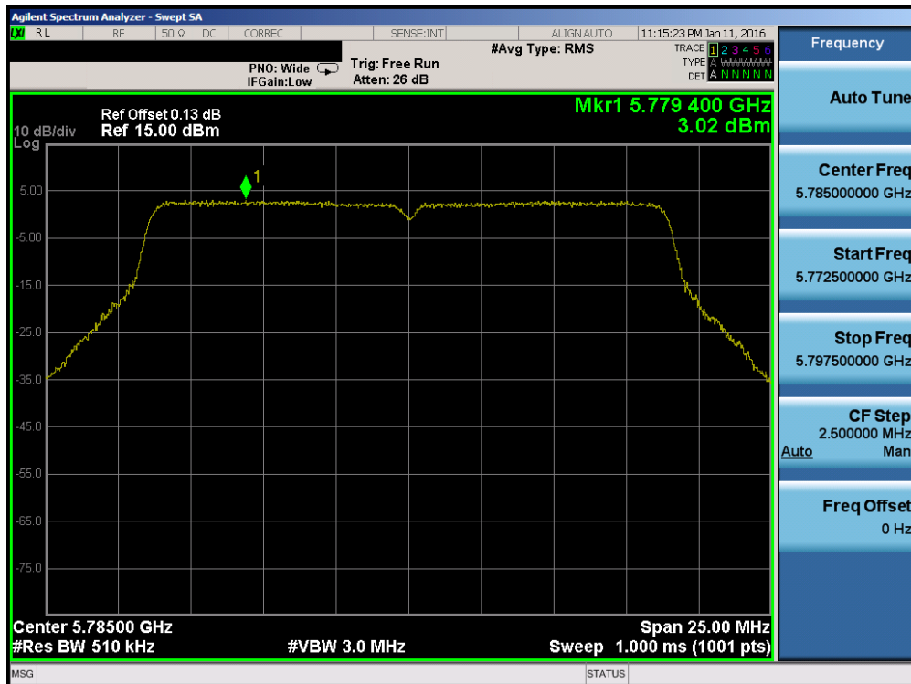
Plot 7-70. Power Spectral Density Plot (20MHz BW 802.11n (UNII Band 3) – Ch. 157)
