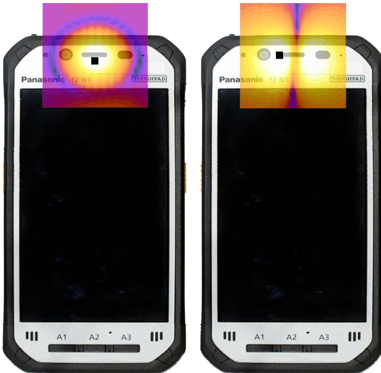
Figure 13-3 T-Coil Scan Overlay Magnetic Field Distributions
