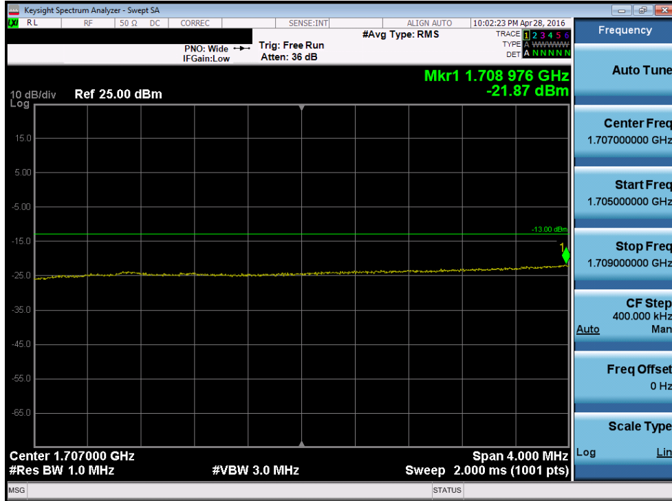
Plot 7-137. Lower Extended Band Edge Plot (Band 4 – 15.0MHz QPSK – RB Size 75)
