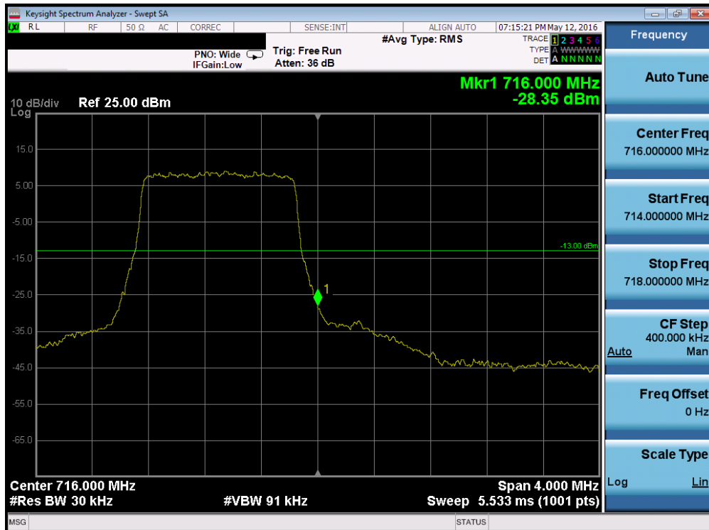
Plot 7-86. Upper Band Edge Plot (Band 12 – 1.4MHz QPSK – RB Size 6)
