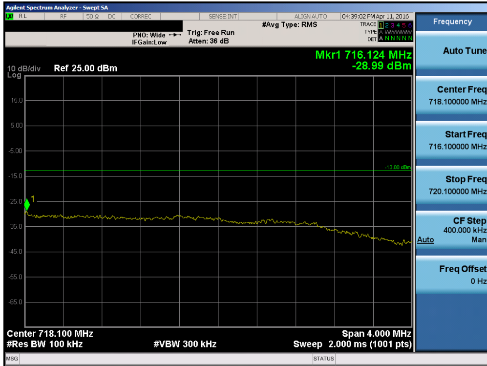
Plot 7-95. Upper Extended Band Edge Plot (Band 12 – 5.0MHz QPSK – RB Size 25)
