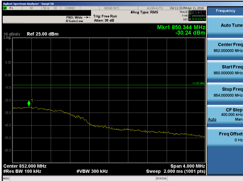
Plot 7-113. Upper Extended Band Edge Plot (Band 5 – Band 5 – 3.0MHz QPSK – RB Size 15)
