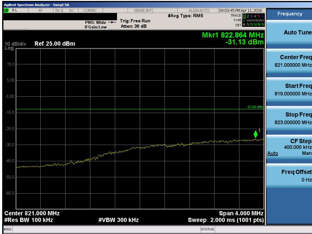
Plot 7-115. Lower Extended Band Edge Plot (Band 5 – 5.0MHz QPSK – RB Size 25)
