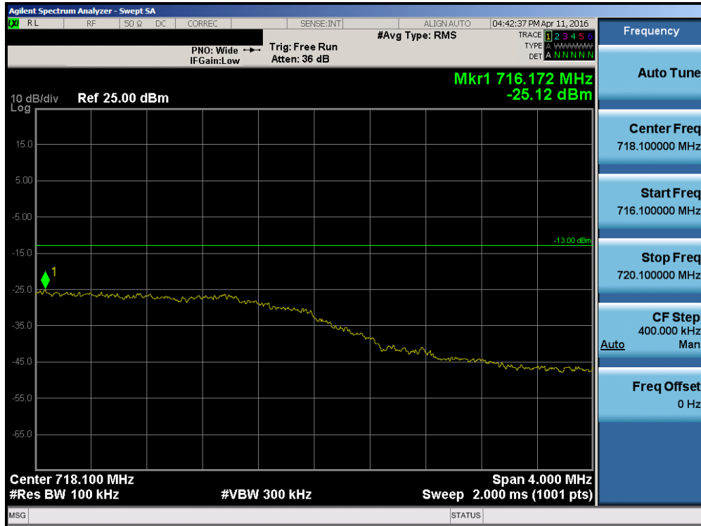
Plot 7-91. Upper Extended Band Edge Plot (Band 12 – 3.0MHz QPSK – RB Size 15)
