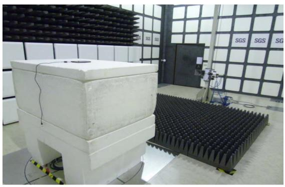
Radiated Emission Set up Photos (Front View)
