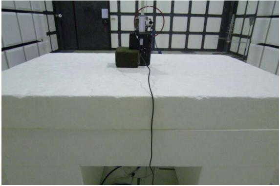
Radiated Emission Set up Photos (Below 1GHz)
