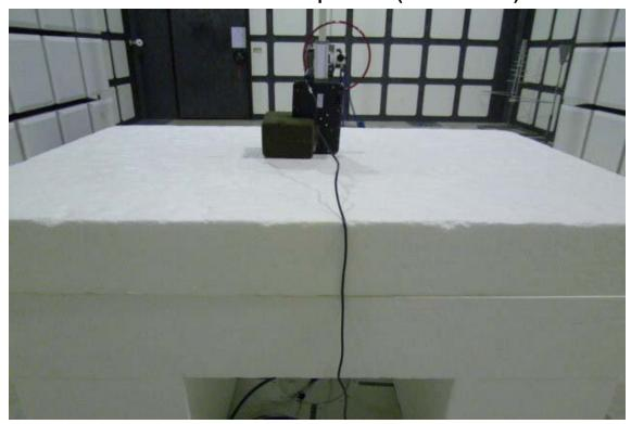
Radiated Emission Set up Photos (Below 1GHz)
