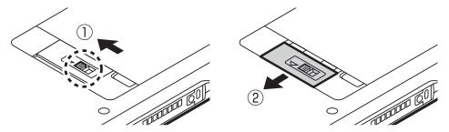
2. Insert your fingertip into the bottom-right groove of the battery (circled in the illustration), lift the battery (1) and then remove it (2).
