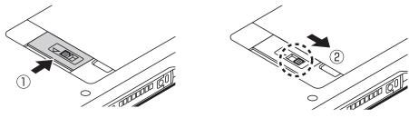
• If the gap above the latch or the red area inside the switch is visible, the latch is not properly closed or locked.
