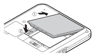
**2.** Press down firmly on the outside edges of the battery to seal it closed.
