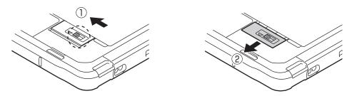
2. Insert your fingertip into the bottom-right groove of the battery (circled in the illustration), lift the battery (1) and then remove it (2).
