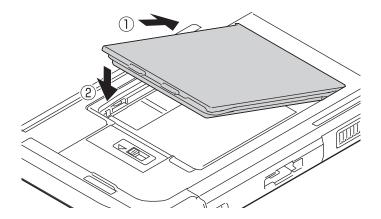
2. Press down firmly on the outside edges of the battery to seal it closed.
