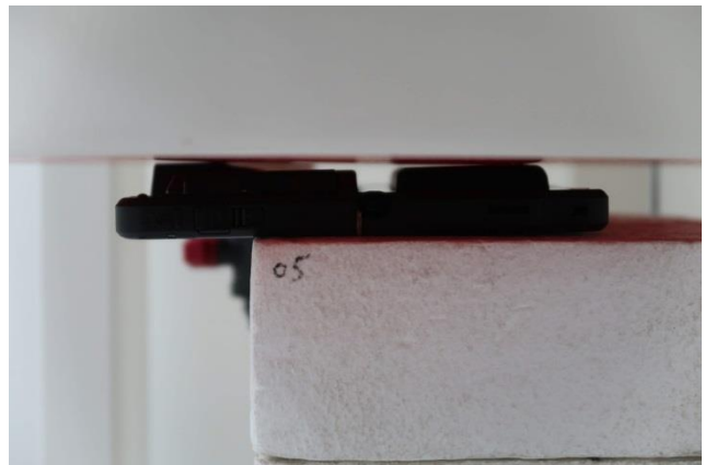
Bottom Face with USB+Battery 2, Test Separation 0 mm
