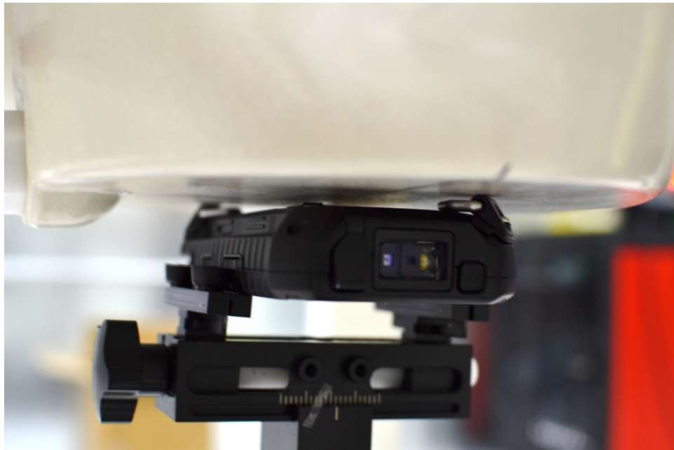
SAR Test Setup Photo 6: Back Side at 0.0 cm with Hand Strap Accessories (Top-Right)
