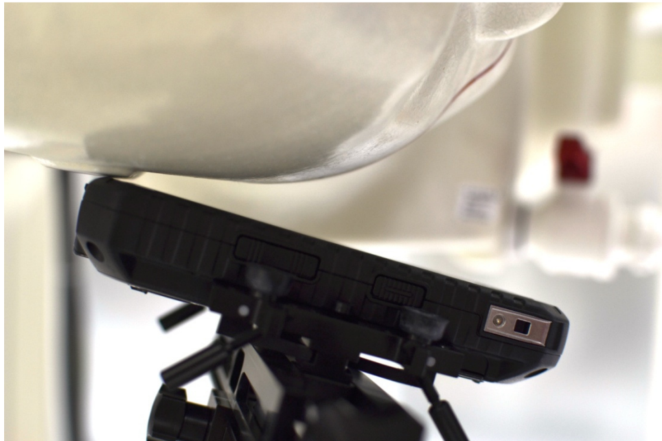
SAR Test Setup Photo 2: Right Tilt
