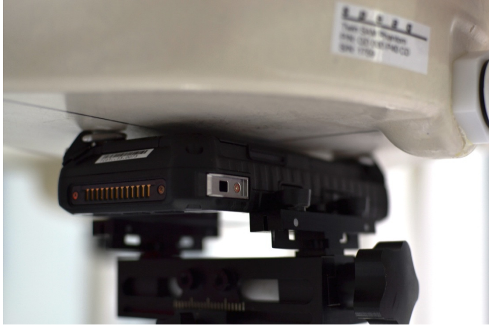
SAR Test Setup Photo 7: Back Side at 0.0 cm with Hand Strap Accessories (Top-Left)
