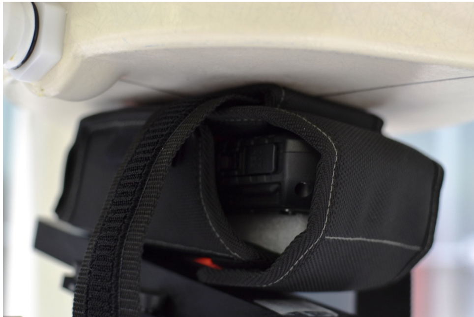
SAR Test Setup Photo 10: Front Side at 0.0 cm with Body Holster Accessory
