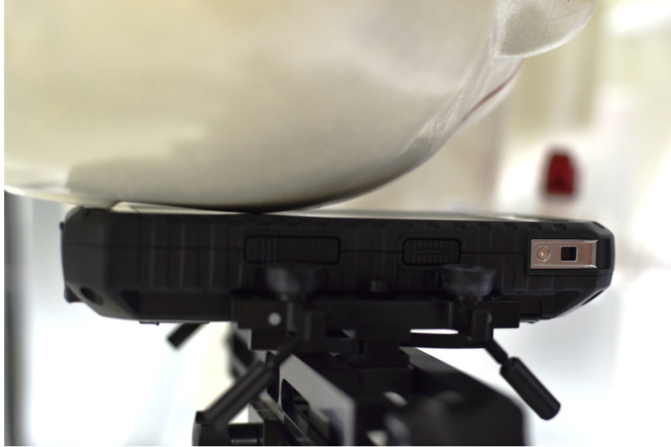
SAR Test Setup Photo 1: Right Cheek
